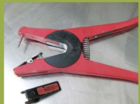
Universal applicator with jaw insert removed
